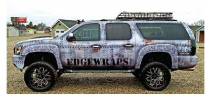
AutoMark<sup>™</sup> vinyl has a surface gloss that has been formulated to match traditional cast vinyl. Our vinyl has an initial surface gloss of > 80 when measured at a 60° observation angle. This is comparable to most white pigmented cast vinyl films used in wrap applications.
